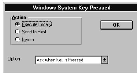
Figure 9-7 Select the Execute Locally option to access the Clipboard Viewer on the remote PC.
